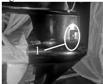
1. Inlet of cooling water channel
