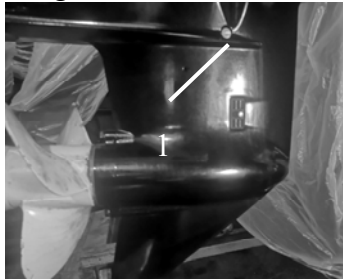
1. Oil level plug screw
