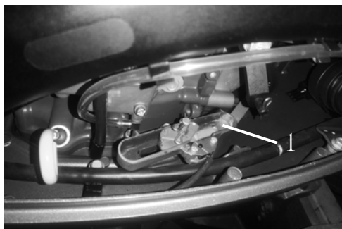
1. Throttle swing rod seat;
